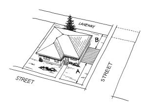
(6) Driveways shall be a minimum of 4.6 metres (15 ft.) from the intersection of two public roadways (as illustrated as setback A on Diagram) and 3.0 metres (10 ft.) from the entrance to a lane (as illustrated as setback B on Diagram).
