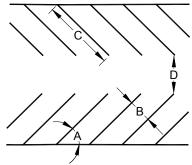
A: Parking Angle C: Depth Of Stall B: Width Of Stall D: Width Of Aisle
